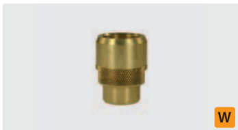
M24 IG : M14x1 IG. Messing. Max. 400 bar
