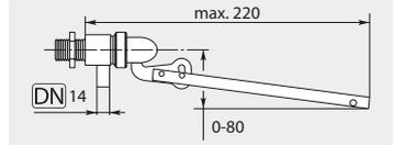
3/8" AG. Messing. Max. 10 bar / 85 °C
